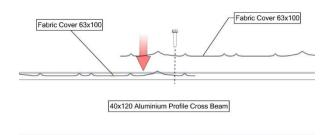
**4.** After installing the ceiling sheets, you can place the side cover profiles.
