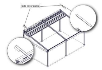
**5.** Wall finish: Before fixing the wall finish profile, apply sealant behind the wall finish profile.
